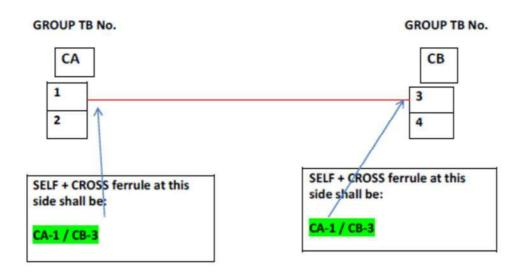
i.e. For nearest Terminal Block no. of cable 1<sup>st</sup> (SELF address) and then "/" 2<sup>nd</sup> (CROSS address) in which Terminal Block no. cable is terminated.
