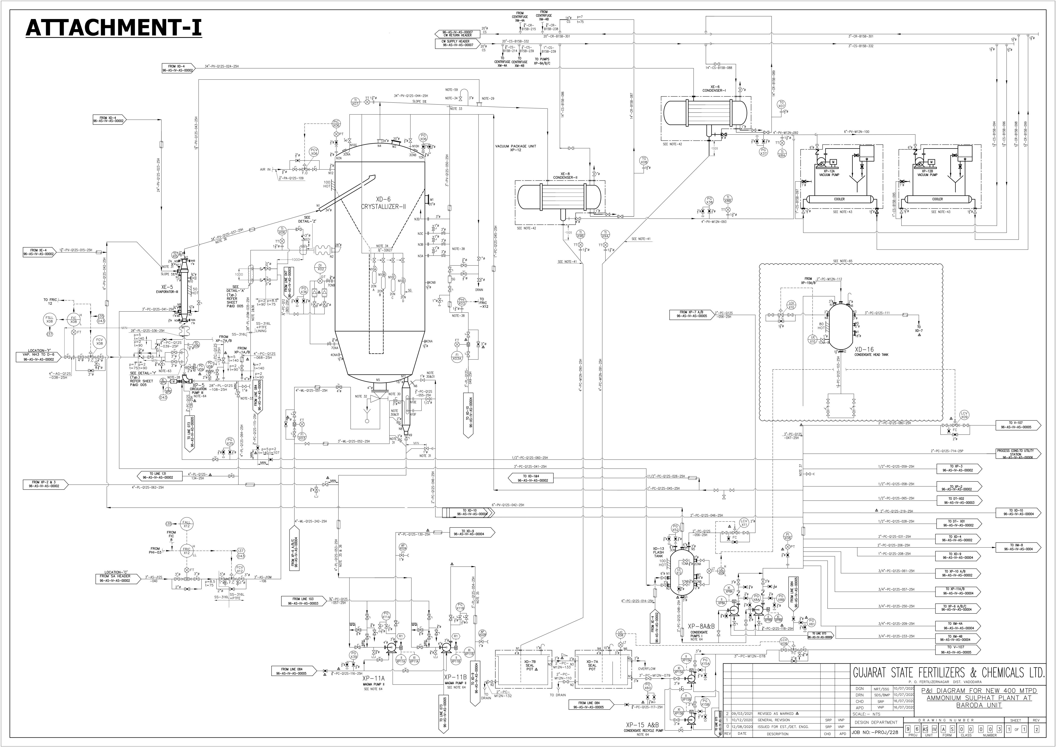
NOTES FOR P&ID NO 96-AS-IV-AS-00002 TO 005: -. OUTLET LINE TO BE PROVIDED WITH NO ELEVATION CHANGE FROM AMMONIA VAPORIZERS (XE-1A/B) TO AMMONIA SEPARATOR (XD-19A/B) 2. PTFE LINING OF 3MM THK. TO BE PROVIDED FROM IN VERTICAL SUCTION PORTION OF XP-2,3,5 OF ~3500MM LENGTH. . INSULATION SHOWN ON PIPES & EQUIPMENTS TO BE OF HOT TYPE MINERAL WOOL / COLD TYPE EPS UNLESS OTHERWISE SPECIFIED.
